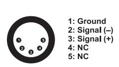
DMX-input XLR mounting-plug:
