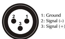
DMX-input XLR mounting-plug:
