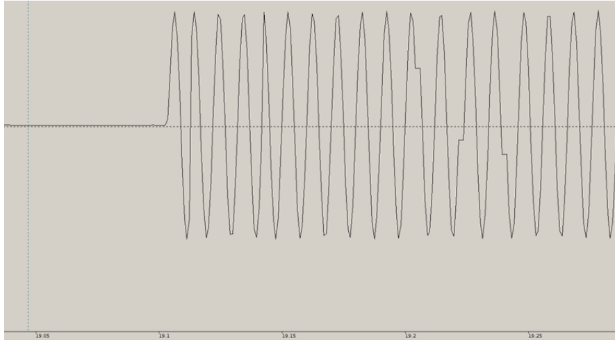
Figure 4.10: Display of acquired bipolar audio signal in OpenViBE indicating latency and distortion
