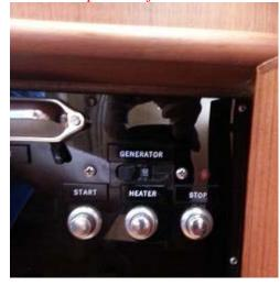
After generator is running, turn your AC power selector switch to generator. Then turn on AC systems as you would on shore power one system at a time.
