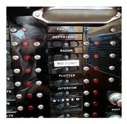
This will power the wash down pump which is located in the forward stateroom under the floor hatch along with the through hull fitting. This system uses sea water not fresh water.
