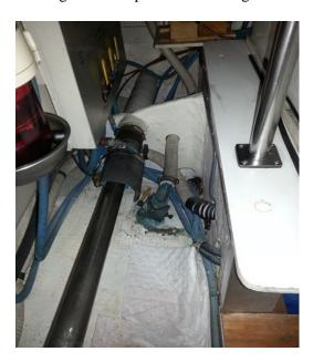
To open the valve, slightly loosen the T handle on the right side of the valve then pull the valve handle upward to a vertical position and re-tighten the T handle.
