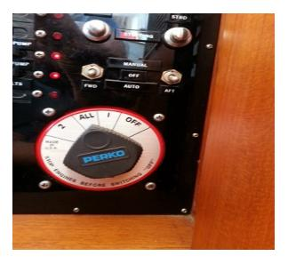
Position #1 is the starboard battery which also has connected to it the small inverter that is used to watch DVD's on the TV or operate the Webasto Heating system. Position two is the Port engine starting battery.
