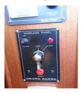
Second release the keeper on the chain tray and if using the foot controls, tap gently on the 'down' foot control to lower the anchor past the roller. When using either helm position use the up/down switches to release or retrieve the anchor.
