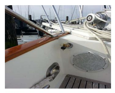
When ready open the faucet valve and begin your cleaning. After you have completed the cleaning of the anchor, close the valve, stow the hose and MAKE SURE you turn the breaker off.
