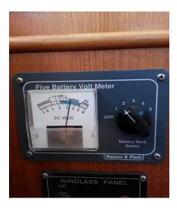
When a battery bank is being charged, the voltage will read from about 13.1 volts to 14.4 volts depending upon state-of-charge of the battery bank. When the battery bank is at rest, (that is, not being charged), the voltmeter can give a rough indication of the state-of-charge of the battery bank.
