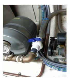
Next open the faucet in the galley sink to relive any pressure in the line. Return to the engine room and using your hands grasp the housing at the top and gently turn the filter housing counter clockwise to remove it.
