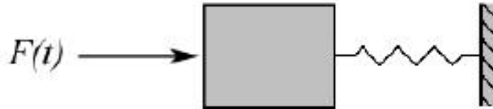
Figure 5.1: 1DOF Spring-Mass System with Friction Damping
