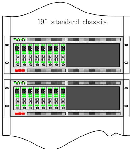
Note: Brackets used to fix the chassis are in the accessory box. If you use the bracket's rear holes to attach brackets to the chassis, there will be 3cm space between chassis front panel and cabinet front panel; and if you use the bracket's front holes, the front panel and the rack will be at the same level vertically.
