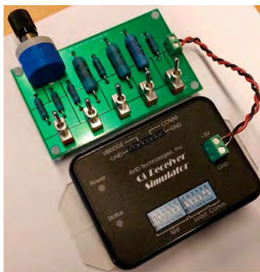
Fig 6. Calibrated Qi receiver simulator with attached variable load (resistor)
