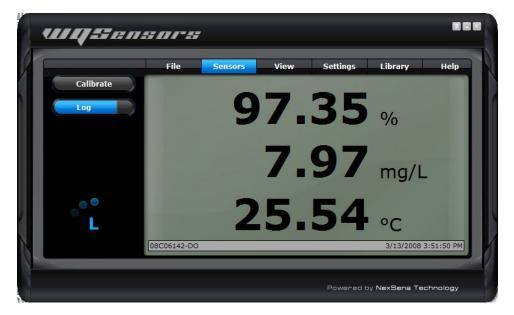
To start logging continuous measurements at the user defined interval, click on the right hand side of the **Log** button. The entire button will turn blue and at the log interval, a short animation with the letter **L** will display on the bottom left hand corner of the screen.
