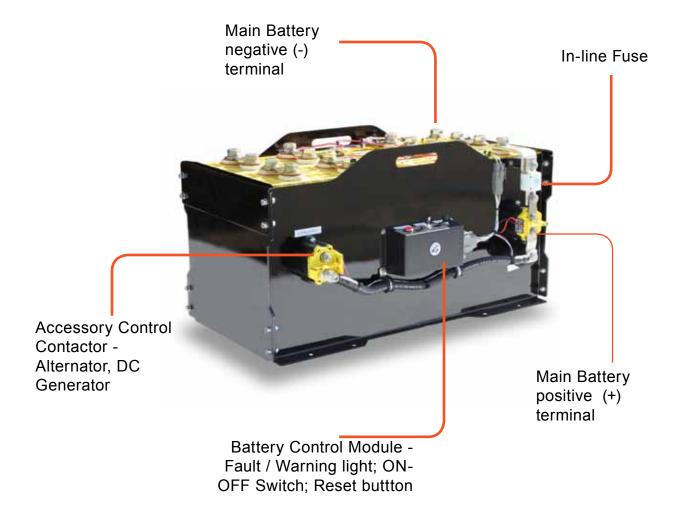
The HIQAP energy storage systems are designed to be connected directly to a Charge controllers and inverter/chargers. ESS systems are shipped with a complete Battery Management System (BMS) and DC contactor controls to protect the battery from over charge, over discharge and over current conditions during daily operations.
