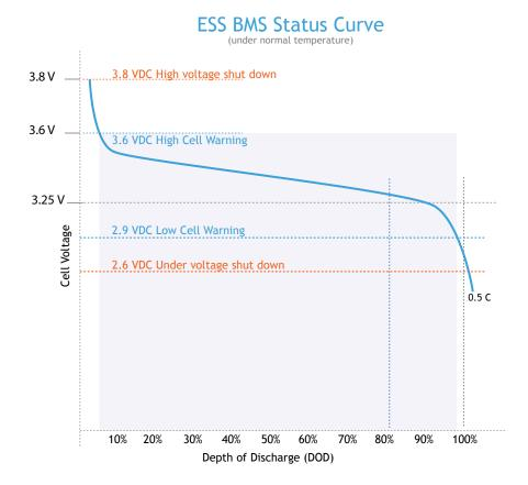
Lithium battery cells used in HIQAP ESS systems have a projected life cycle well in excess of 3,000 cycles at 70% depth of discharge which is estimated to be about four times the life of a conventional deep cycle lead acid battery. The key to achieving this performance is to ensure that each individual cell is protected from being over-charged or over-discharged during daily operation. Listed below are key functions built into the ESS system to ensure battery protection:
