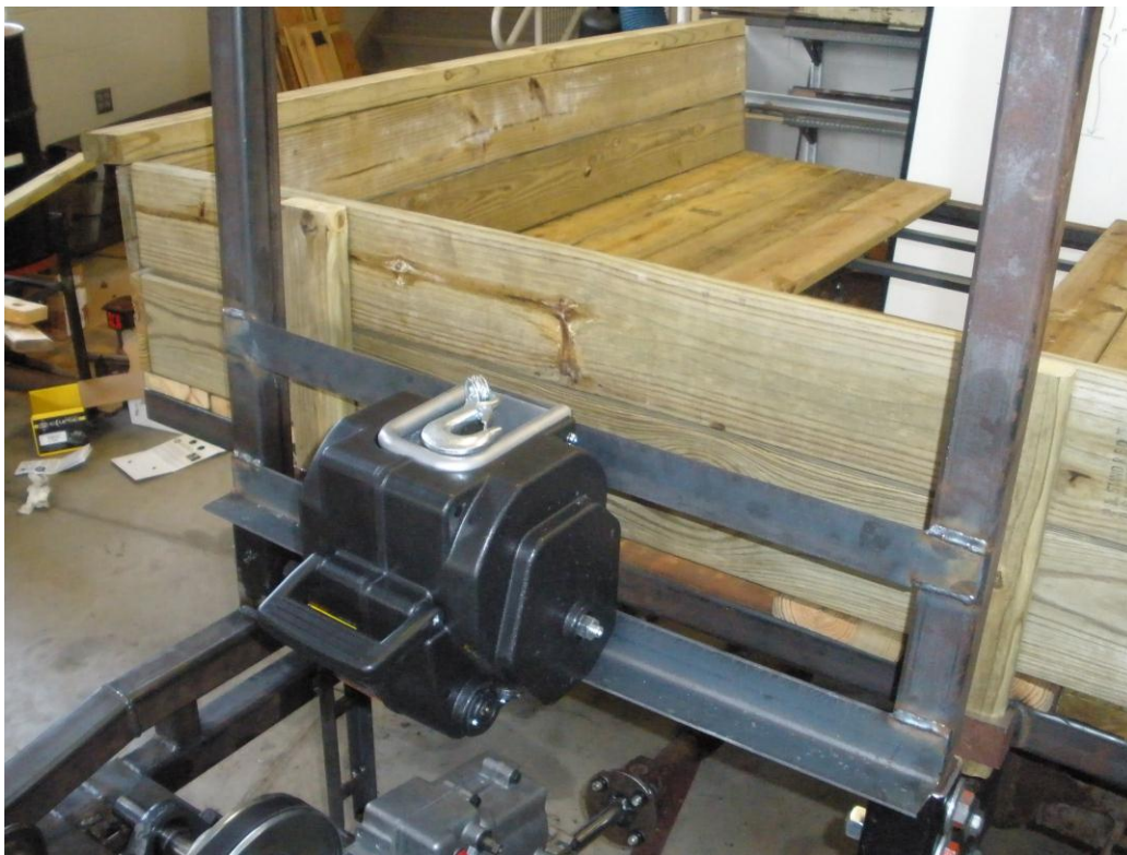
Figure 12: Winch Mounted to Roll Cage
