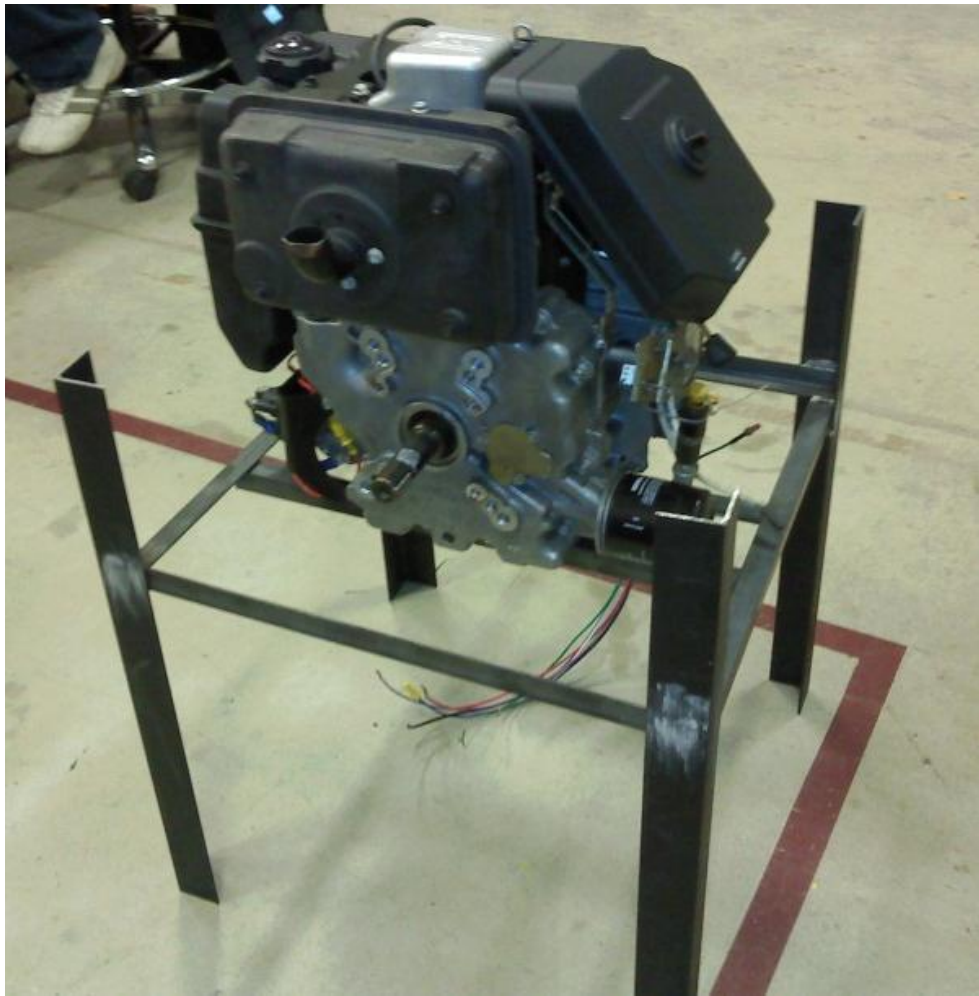
Figure 28: Engine Mount for Testing
