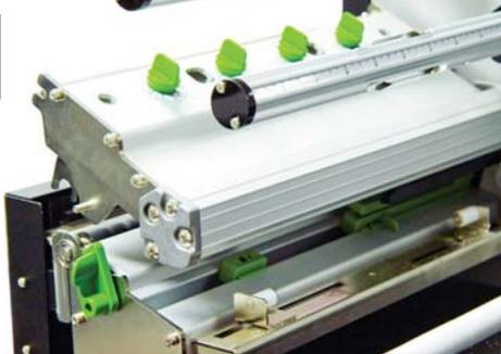
TURN OFF VnM 8 SignMaker, open the VnM8 & lift green lever to open printing assembly.
