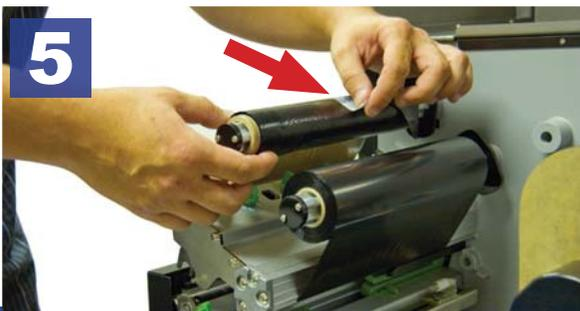
Feed the rear ink roll up to the take up core & attach in the center using a thin adhesive tape.
