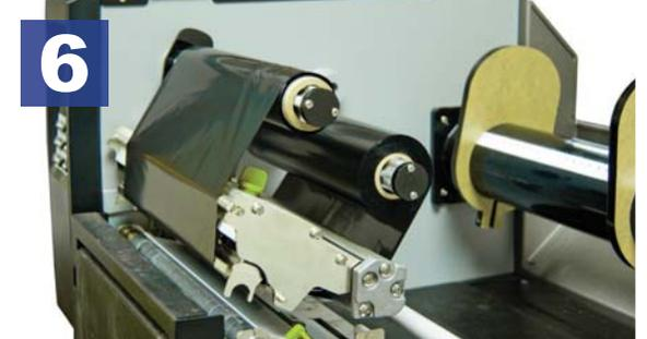
Once attached hand wind the front ink roll spindle up to remove any creases and to keep the tension taut.
