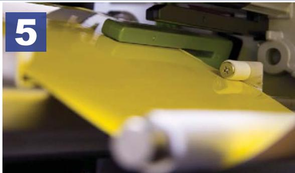
Secure the white media guides to the media and feed under green media sensor bar.
