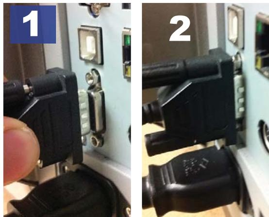
1. Connect the VnM8 Keypad cable (male) to the back of the VnM<sup>®</sup>8 SignMaker port (female).
