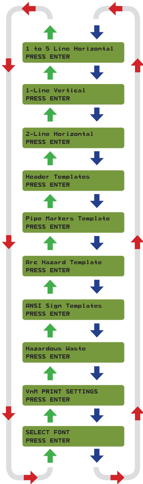
The VnM®8 template navigation tree to the left displays the flow and order of the templates.
