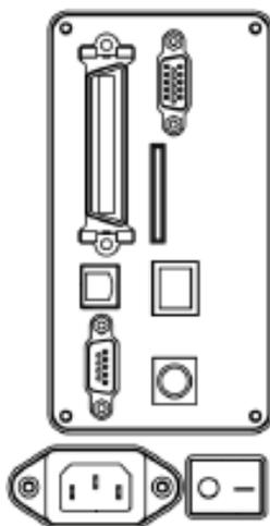
1. After connecting the VnM<sup>®</sup>8 Keypad to the VnM<sup>®</sup>8 SignMaker, connect power cord to the back of the VnM<sup>®</sup> SignMaker
