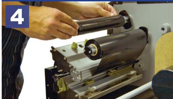
Attach and center the take up core to the front ink spindle.
