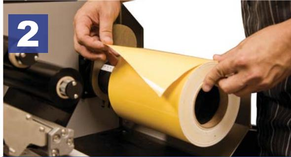
Slide on the VnM8 Media onto the center of the rear Media Spindle
