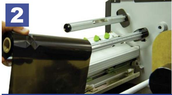
Slide on VnM8 Ink Roll to rear Ink Roll spindle.
