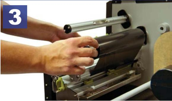
Center the ink roll on the ink roll spindle and feed the ink roll under the printing assembly
