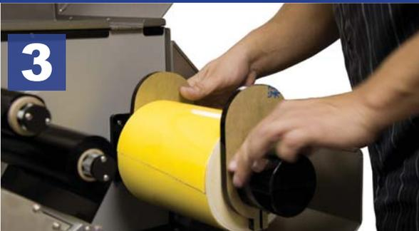
Slide the Media Spindle end guide onto the Media Spindle to secure the VnM8 Media Roll
