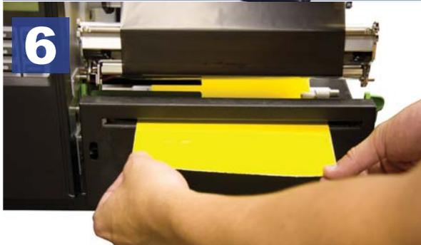
Continue to feed the media under the printing assembly & between the cutter gap.
