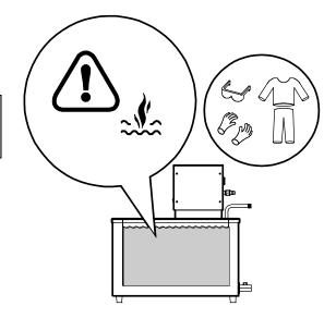
When removing bath fluid do not inhale toxic vapor. Always use appropriate ventilation.
