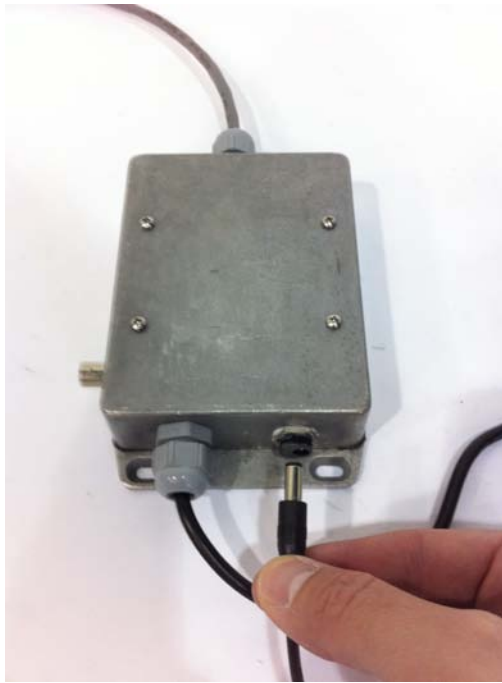
Figure 2: Connecting the 12VDC power supply
