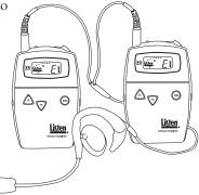
The LA-273 has a uni-directional pick-up pattern. This means that the microphone's element must be oriented towards your mouth. It will not pick up audio very well from the side of the microphone. The main advantage of this type of microphone is that it helps minimize feedback and picks up less environmental noise.
