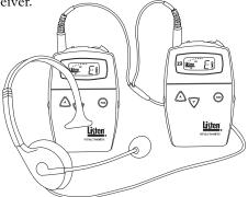
The LA-272 has a uni-directional pick-up pattern. This means that the microphone's element must be oriented towards your mouth. It will not pick up audio very well from the side of the microphone. The main advantage of this type of microphone is that it helps minimize feedback and picks up less environmental noise.
