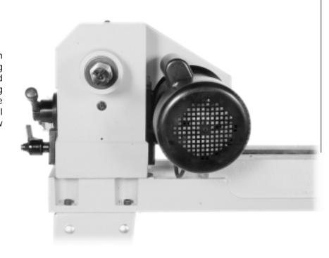
If you are not using the stand place the lathe onto a suitable, sturdy work bench with the headstock to your left, again taking care not to trap the cable. Bolt down securely with suitable bolts.
