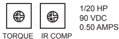
Figure 8. Recommended TORQUE and IR COMP Settings (actual settings may vary with each application)
