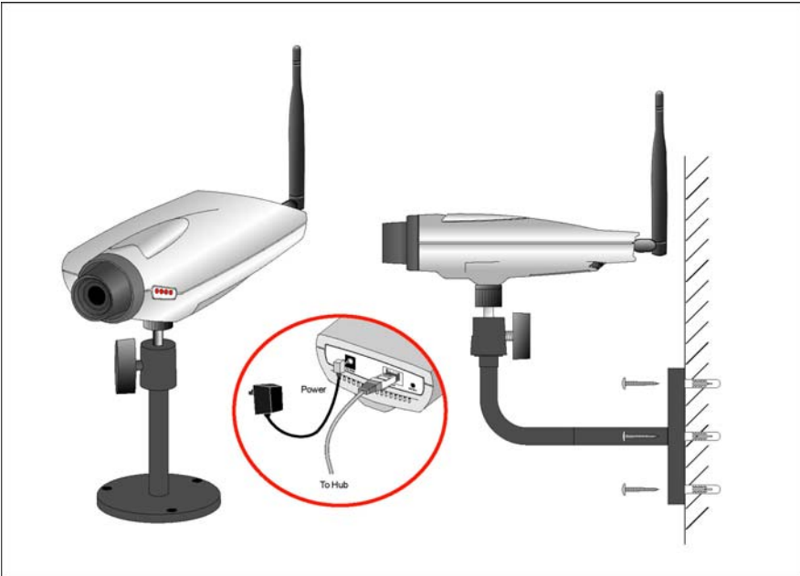
Figure 3: Wireless/Ethernet Network Camera Installation
