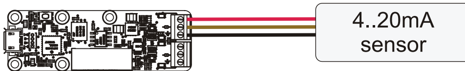
Wiring for a 3 wire sensor, powered by the Yocto-4-20mA-Rx (max. 80mA in all).
