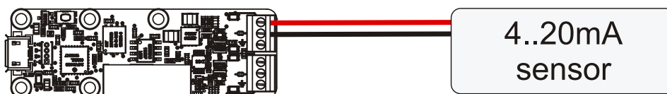
Wiring for a 2 wire sensor, powered by the current loop.
