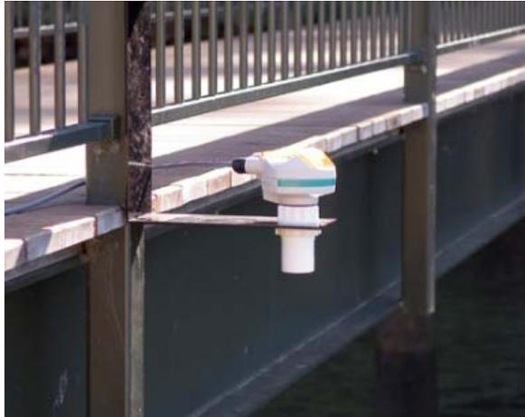
Figure 14: Probe mounting bracket
