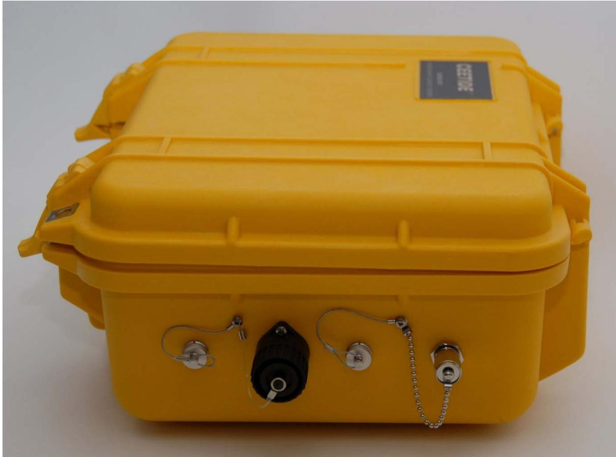
**Figure 2: The connections on the right hand side of the CEETIDE™ control unit**
