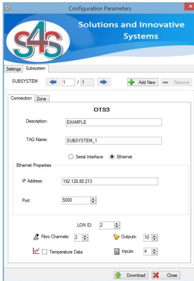
Image 17 Configuration - SUBSYSTEM Connection
