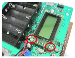
Bolts for LCD, need to be loosened when replacing the spacer (when using different type of motor).
