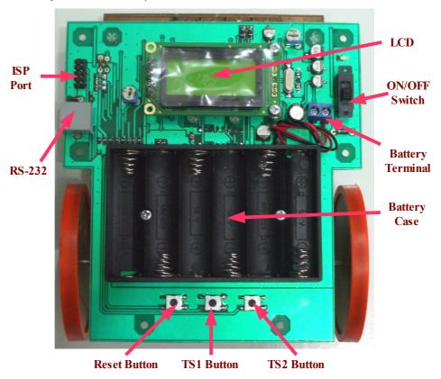
At the time DT-ROBOT LINE FOLLOWER BASE was first turned on, LCD will show a **Tracking Menu** marked with the string "**READY**" on the bottom line and digital combination of sensors reading value on the top line.
