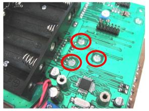
Bolts for castor (upper), need to be loosened when replacing the spacer (when using different type of motor).
