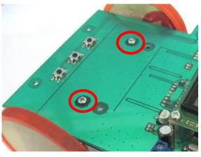
Bolts for bracket (under battery case), need to be loosened when replacing the bracket (when using different type of motor).
