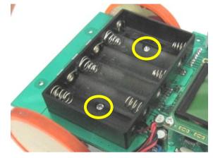
Bolts on battery case, need to be loosened when replacing the bracket (when using different type of motor).
