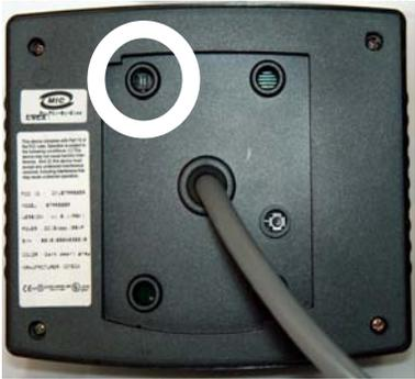
**Figure: DIP Switch location**
