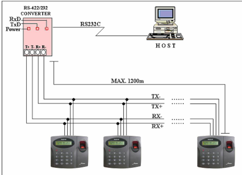
**Figure: RS422 Communication between FINGER006s and the Host PC**
