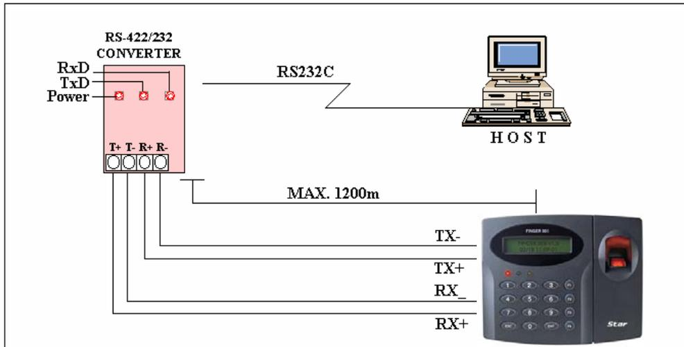
**Figure: RS422 Communication between FINGER006 and Host PC**
