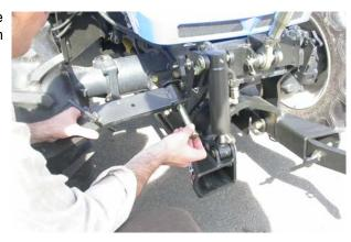
9.6 Loosen and remove the wing nut from the support and vertically position the arm on the support. Maintain the arm and tighten by using the wing nut.
