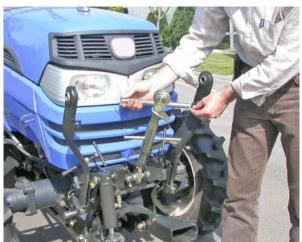
6.3 Support the L.H. arm and loosen the wing nut.
