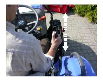
**12.2.2** Controlling the auxiliary hydraulic line (depending on the fittings). Move the MX monolever to the right and left.
