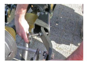
Adjust the locknut to ensure the locking point.
