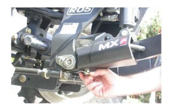
9.5 Position the arm on the R.H. side support of the front linkage using the pin and the locking pin (pay attention to the direction of the arm when handling it).
