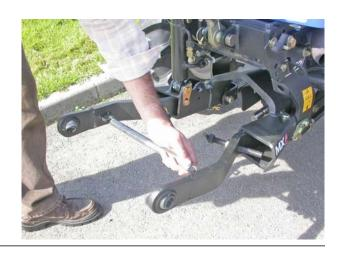
9.4 Remove the locking pin and pin to free the R.H. arm.
