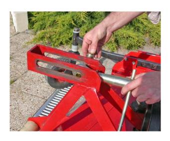
7.6 Replace the locking pin as shown opposite. The hook therefore remains in open position when the front linkage is being used.
