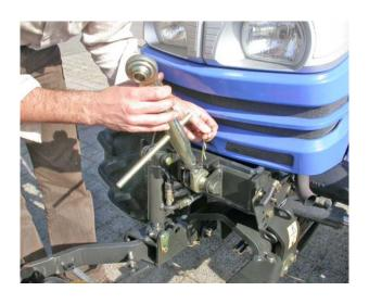
Hitch the top link bar to the mast of the front implement.
