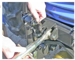
7.7 .Set the length of the top link bar to obtain the required movements from the front implement. Lock the adjustment of the bar by means of the lever locknut.
