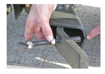
.Support the top link bar and remove the locking pin. 7.4
