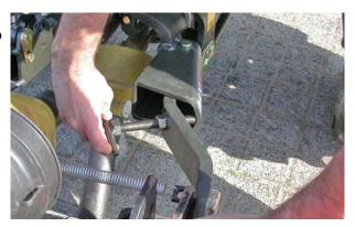
**8.5** Tighten the adjustment screws of the arms.
