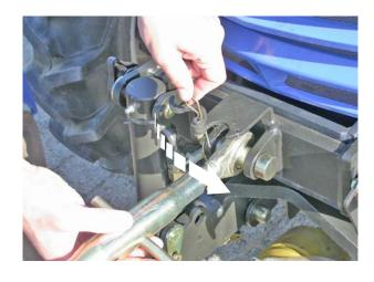
**8.4** Loosen the adjustment screws of the arms so as to be able to unhitch the implement.
