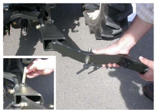
6.5 Insert the locking pin into the pin.
