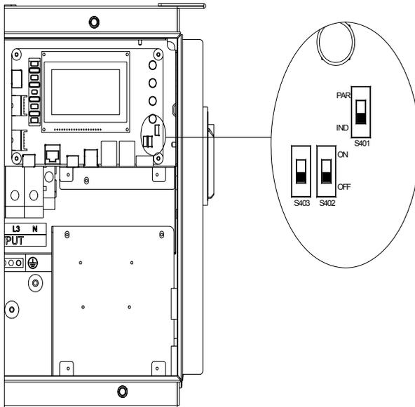
Figure 3-22 Location of the PV connection mode selector switch
