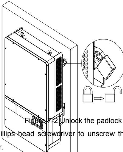
b.) Use a No.2 Phillips head screwdriver to unscrew the 2 screws on both sides of the inverter.
