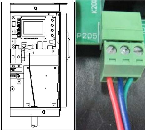
Figure 3-36 The dry contact communication cable connection
