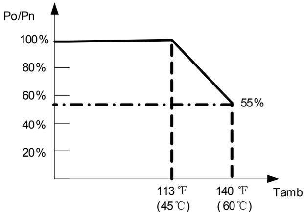
Figure 8-2 SCA36KTL derating curve with high temperature
