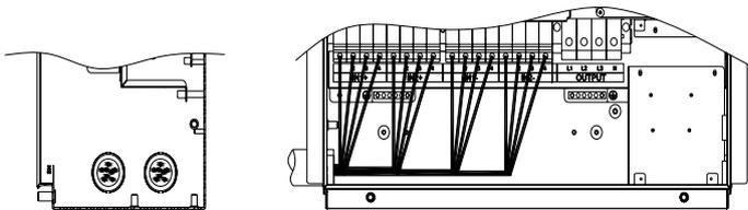
Figure 3-25(b) Connection of DC input cables
