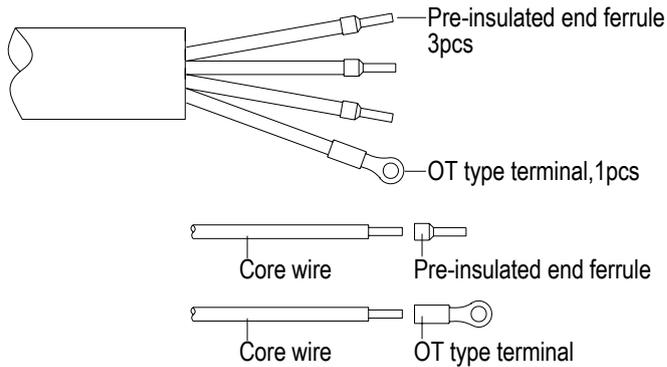
Figure 3-29 AC output and ground cable set up
