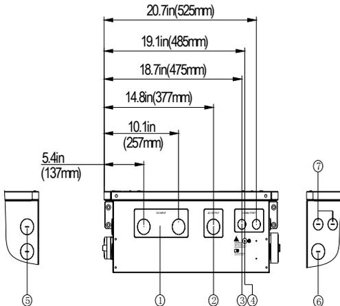
Figure 3-18 External connection ports
