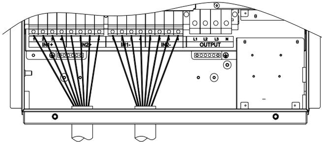
Figure 3-25(a) Connection of DC input cables
