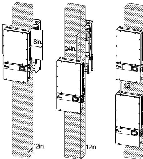
Figure 3-4 Inverter pillar mounting dimensions
