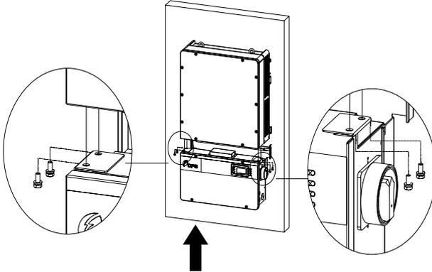
Figure 3-11 Installation of the wiring box
