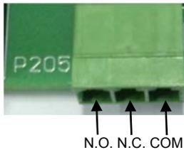
Figure 3-32 Dry contact communication port
