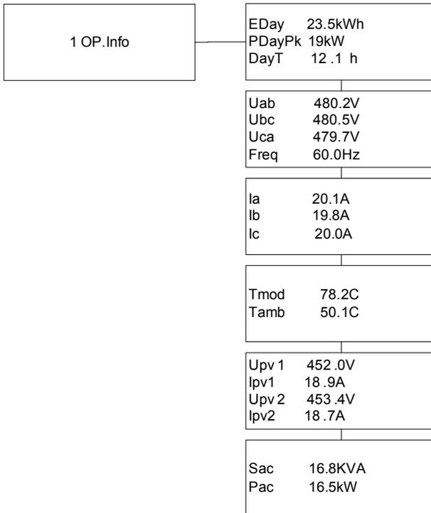
Figure 5-8 Operation information indication (PV independent mode)
