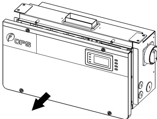
Figure 3-16 Take off the cover of the wiring box
