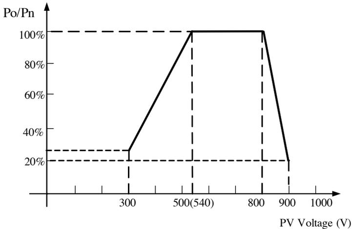
Figure 8-1 SCA36KTL derating curve of PV input voltage
