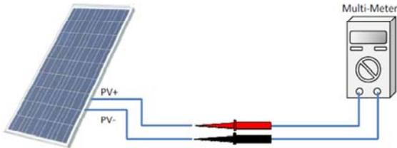
Figure 3-23 Polarity check
