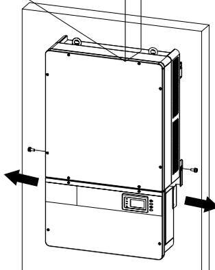
Figure 7-3 Remove the screws on both sides
