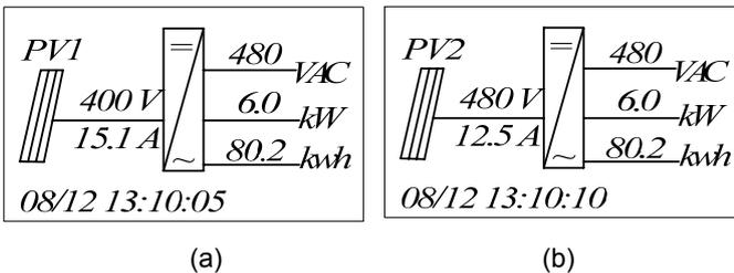
Figure 6-2 Default indication interface for normal operation
