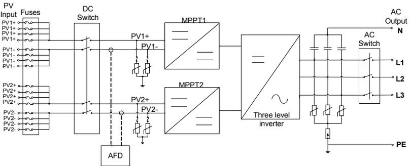
Figure 2-2 Schematic diagram of CPS SCA36KTL-DO/US inverter
