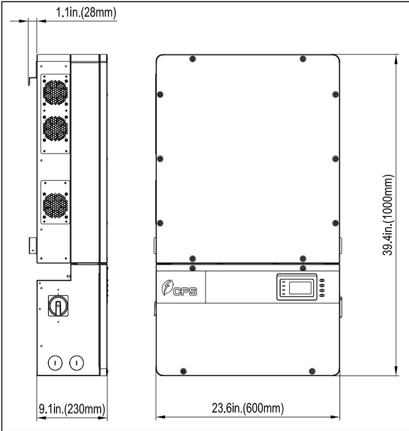
Figure 3-1 Dimensions of CPS SCA36KTL-DO/US inverter
