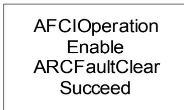
Figure 5-21 Manually clear “ARC Protect” fault
