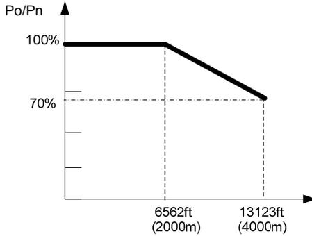
Figure 8-3 SCA36KTL derating curve with high altitude
