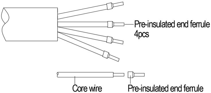
Figure 3-28 AC output and ground cable set up
