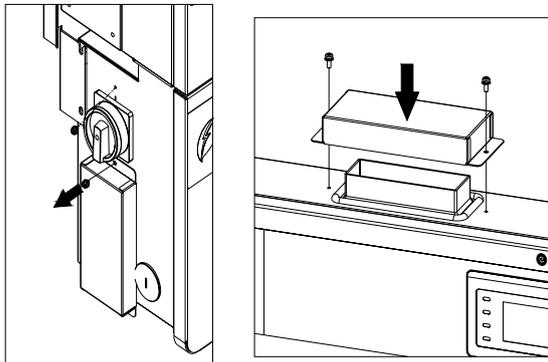
Figure 7-5 Install the cover board on the connector of the wiring box
