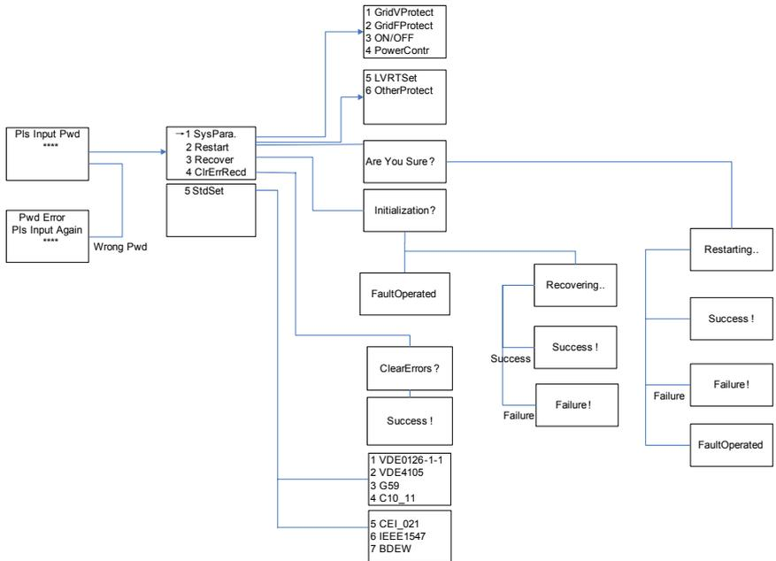
Figure 5-14 System protection parameter configuration
