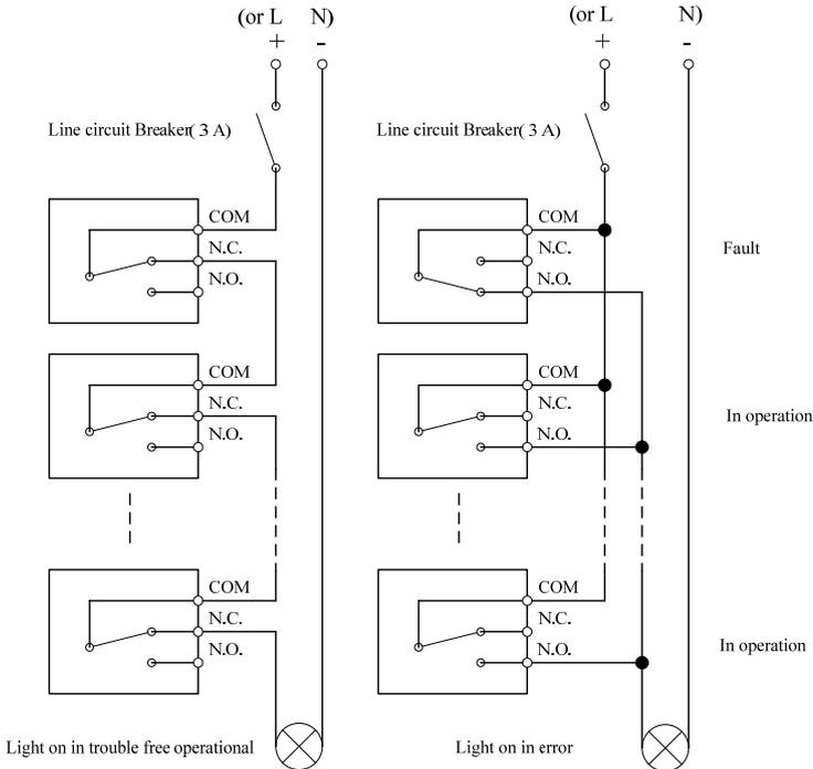
Figure 3-33 Schematic diagram of dry contact communication
