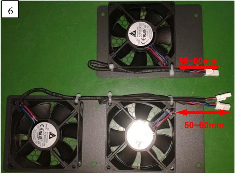
Figure 7-1 Replace cooling fans
