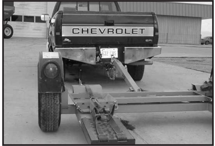
**Step 13.** To pull the **TOW-IT** empty, make sure tie-down straps are tightened in the storage position, and towed vehicle safety chains are wrapped up and hooked. Tie-down winch handles should be left in a down position (horizontal) with safety pins in place when towing loaded or empty. **DO NOT ATTEMPT TO PULL TOW-IT WITH WHEEL PLATFORM IN LOADING (tilted) POSITION.**
