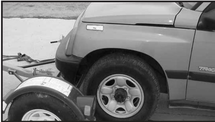
**Step 5.** With someone safely guiding you, slowly drive vehicle onto platform **FRONT FORWARD**. (Any vehicle mounted on tow dolly must be mounted with front of the vehicle facing forward.) Drive the car forward until the tires touch the ramps. Make sure the tire is aligned to ascend onto the ramps.
