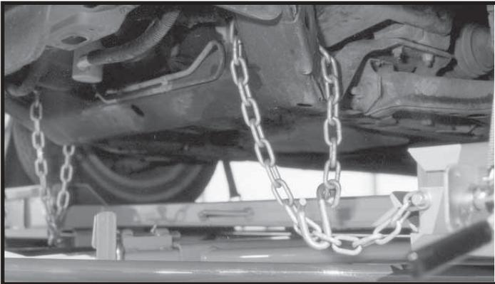
**Step 11.** Hook the towed vehicle safety chains to frame of vehicle directly above the area where the chains are mounted on the **TOW-IT**. Leave some slack in the chains to allow suspension movement of the towed vehicle. **Review the safety points on page 1 before moving vehicles.**
