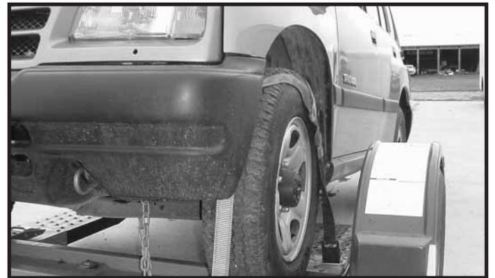
**Step 8.** Be sure tie-down winch is centered with the tire before tightening straps.
