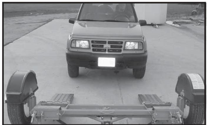
**Step 4.** Before loading (and unloading) towed vehicle make sure platform and towed vehicle are in straight alignment. Tow dolly must be completely and properly hooked up to the towing vehicle. **Towing vehicle must be larger and at least 1000 lbs. heavier than the tow dolly and towed vehicle combined.**
