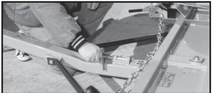
2) Pull locking pin toward the hitch as far as it will go. The wheel platform will tilt back to allow loading.
