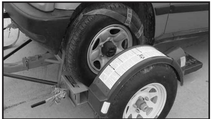
**Step 9.** While tightening straps, pull cross strap forward to ensure even tightening. Tighten straps until each tire starts to flatten against tire stop. After each strap is tight, insert a safety pin in each winch. Disengage towed vehicle parking brake.
