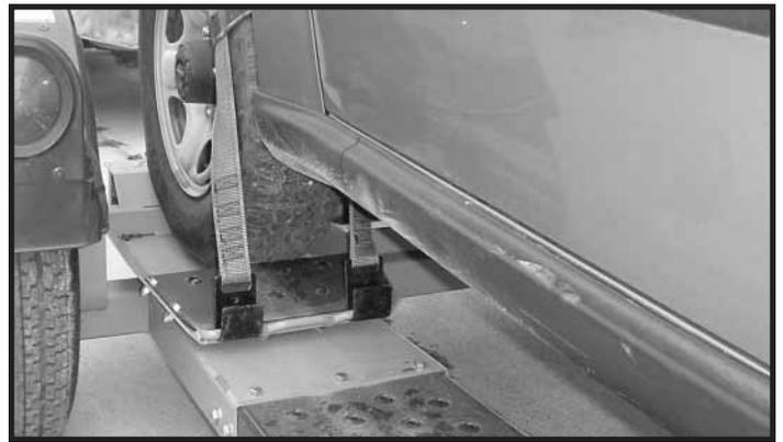
**Step 7.** Place one tie-down strap over each tire and secure hooks to rods located at the rear of each wheel platform. The short side of the hook must face the rear of the **TOW-IT**.
