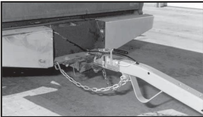
**Step 1.** Secure ball coupler to 2" (3,500 lb. capacity) towing vehicle ball only. Make sure that the hitch and the hitch ball are in good condition and not rusted, loose or stripped. **Recommended ball height is 18" to the top of the ball.** Make sure hitch is locked down and secured with safety clip. Criss-cross safety chains under tongue and secure to towing vehicle frame.
