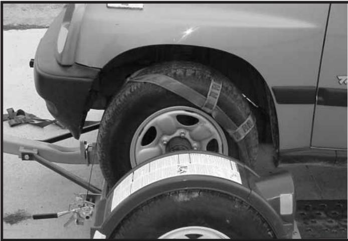
**Step 10.** Make sure the tie-down strap is the correct size for the auto tire. The picture above shows a correct fitting strap. See page 1 of this instruction for proper fit and exchange instructions.
