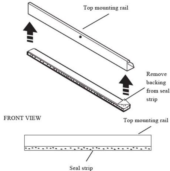
2. Attach the top rail onto the top of the outer case using the four 2/5" screws.
