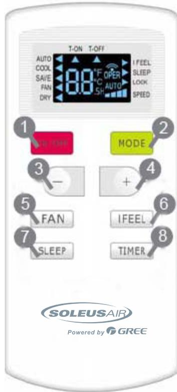
9. **LOCK/UNLOCK** - Press the “+” and “—” buttons simultaneously to lock and unlock the remote control. When the remote is locked, none of the functions or setting can be changed using the remote.
