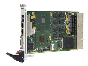
Equipped with the Intel® high-performance Core 2 Duo processor T7500 running at 2.2 GHz, the F18 is a versatile 4HP/3U (single-slot, single-size Eurocard) single-board computer based on the latest multi-core processor architecture from Intel® with full 64-bit support. The board delivers an excellent graphics performance and is designed especially for embedded systems which require high computing performance with low power consumption.
