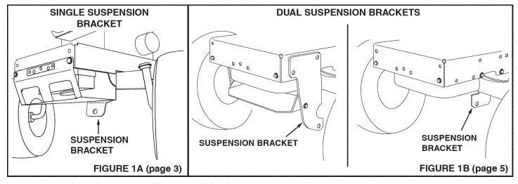
Look under the front of your tractor (Figure 1A & 1B). If there is a single mower deck suspension bracket located underneath the middle of the front axle, continue on to INSTRUCTIONS FOR SINGLE SUSPENSION BRACKET TRACTORS on page 3. If your tractor does not have a mower deck suspension bracket underneath the middle of the front axle, skip to INSTRUCTIONS FOR DUAL SUSPENSION BRACKET TRACTORS on page 5.
