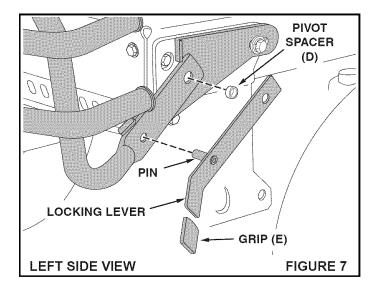
3. Fasten locking lever and bumper to mounting bracket using a screw (A) or bolt (B), a lock washer (F) and a flat washer (G). Use screw (A) for LT tractors and bolt (B) for GT tractors. Assemble screw or bolt through pivot spacer in rear hole in bumper and into tractor frame. Tighten. Repeat for other side.
