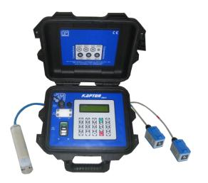
With **KAPTOR MULTI** B.M. Tecnologie Industriali developed and introduced in water flow Measurement Market the first multi-purpose Data Logger for measurement in full pipes and open channels. **KAPTOR MULTI** is a Data Logger developed for measuring in water networks, aqueducts and sewerages. Depending on the applications, it can be equipped with the module **TTFM KAPTOR** or **OCM KAPTOR**.
