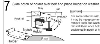
For some vehicles with fatter rails, it may be necessary to completely remove knob and washer and reinstall them once bolt is positioned in notch of holder.
