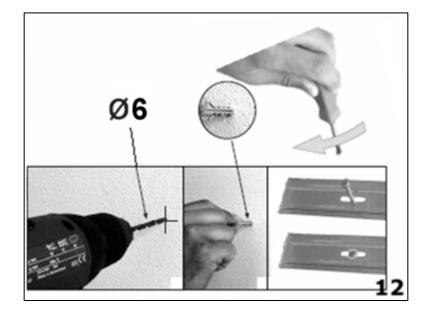
**12)** Using a 6 mm drill bit, drill out two holes on the pencil markings that you made in step 11. Insert rawl plugs into the holes and then use a screwdriver to secure the fixing bracket to the wall.
