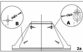
**2a)** The support screw holes are indicated by figure  $\boldsymbol{A}$  in this drawing and the anchoring screw holes are indicated by figure  $\boldsymbol{B}$ .
