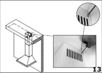
o Slide chimney section **(D)** inside of chimney section **(C)**. Then secure the L shaped bracket to the wall, using the same method as you have just used to secure the lower bracket.
