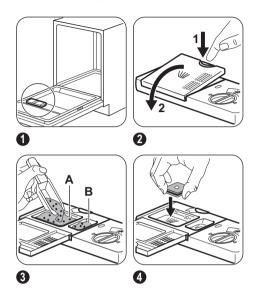
Put the detergent or the tablet in compartment (A) If the programme has a prewash phase, put a small quantity of detergent in compartment (B).
