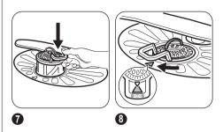
To remove filters (**B**) and (**C**), turn the handle counterclockwise and remove. Pull apart filter (**B**) and (**C**). Wash the filters with water. Remove filter (**A**). Wash the filter with water. Before you put the filter (**A**) back, make sure that there are no residues of food or soil in or around the edge of the sump.
