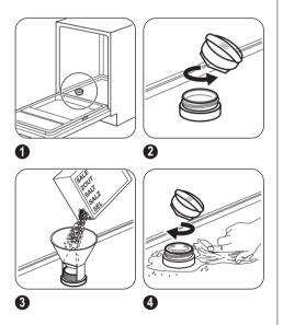
Put 1 litre of water in the salt container (only for the first time).
