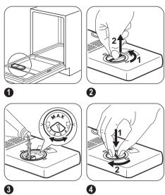
To adjust the released quantity of rinse aid, turn the selector between position 1 (lowest quantity) and position 4 (highest quantity).
