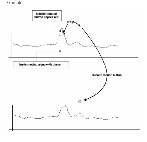
Fig. 53 Moving the measuring cursor to a different peak (signal curve zoomed in 3 times)
