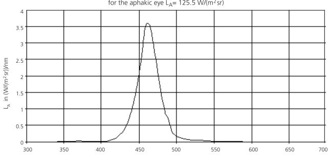
Photochemical radiation density of a light source (white LED - slit illumination) for the aphakic eye  $L_A$ = 125.5 W/(m<sup>2</sup>sr)
