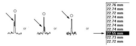
Such measuring curves or measurement series require immediate verification, either between individual measurements (in ALM mode) or in post-run editing (without the patient in front of the device). Interpretation or post-run editing should always be performed with the help of the zoom function!
