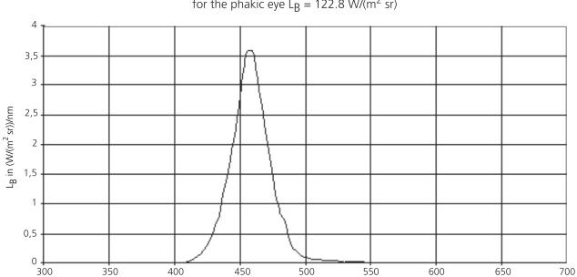
Photochemical radiation density of a light source (white LED - slit illumination) for the phakic eye  $L_B = 122.8 \text{ W/(m}^2 \text{ sr})$
