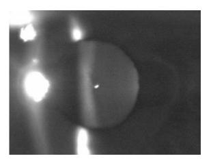
Fig. 74 Reflection in corneal image due to lateral misadjustment
