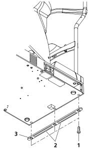
Fig. 7 Mounting holding bracket
