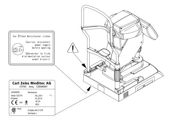
Fig. 1 Warning and information labels on the device
