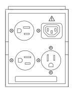
Fig. 6 Power isolation transformer, output side 120 V
