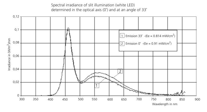
"Optical axis" or "0°" corresponds to the direct view into the illuminating projector. 33° is the angle for the intended use in anterior chamber depth measurement.
