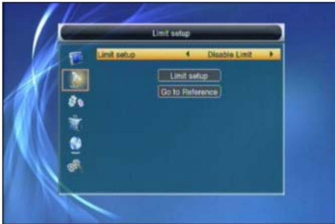
1 When you set "limit setup" to "West Limit/ East Limit", you can move the highlight to "Limit Setup" line and move the dish to west or east by pressing [Left/Right] key manually.
