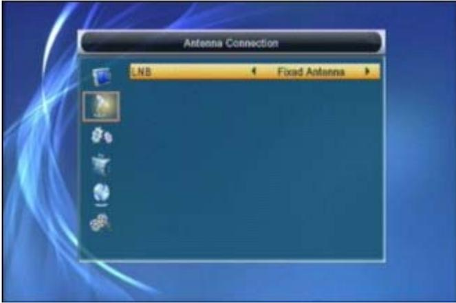
Press [Left/Right] key to select LNB. Option: Fixed Antenna / Motor Antenna.
