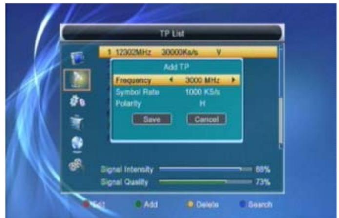
4 Press [Yellow] key will open dialog box asking you whether confirm to delete current TP. When select "Yes", you will delete the channel which highlight focus on. When select "No", it will cancel the operation.
