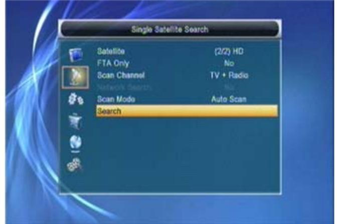
1 In "Satellite" item, press [Volume Up/ Volume Down] key to select satellite, which you to scan. Otherwise, press [OK] key can open the "satellite list" for you to select directly.
