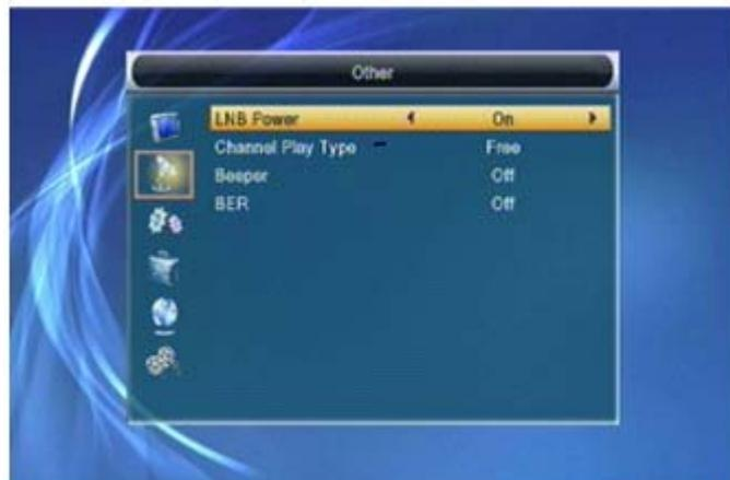
1 In "LNB Power", there are two options, "On" and "Off", for your selection. If the setting is "On", the receiver will supply power to satellite antenna. If the setting is "Off", the receiver won't supply power to satellite antenna.
