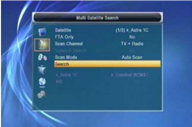
1 In "Satellite" item, press [Enter] key to see the selected satellite. The system will use DiSeqC1.0 / DiSeqC1.2 / USALS function to search satellite and scan channels. It will scan all the satellite displaying in the bottom box.
