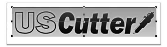
With the image selected, select "Monochrome – 1 bit" from the Mode section of the Image drop down menu.
