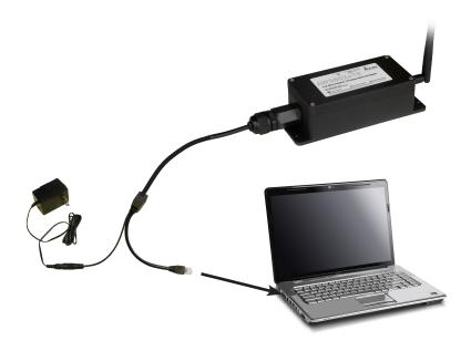
Step 3. The default IP address of the radio is written on its product label. This default address is usually 192.168.17.17. The default login password is "password." You must configure your PC's wired LAN port to the same subnet and an IP address different from this one. With this configuration in place, you should be able to use a web browser on your PC to log in to the radio's interface.
