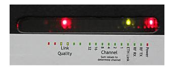
**Status LEDs:** The top cover of each radio provides a window showing status lights with a legend on the product label:
