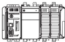
In a 1769-L3x controller system, the 1769 I/O modules can be placed to the left and the right of the power supply. As many as eight modules can be placed on each side of the power supply.
