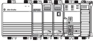
The 1768-L4x controller combines both a 1768 backplane and a 1769 backplane. The 1768 backplane supports the 1768 controller, the 1768 power supply, and a maximum of four 1768 modules. The 1769 backplane supports 1769 modules.
