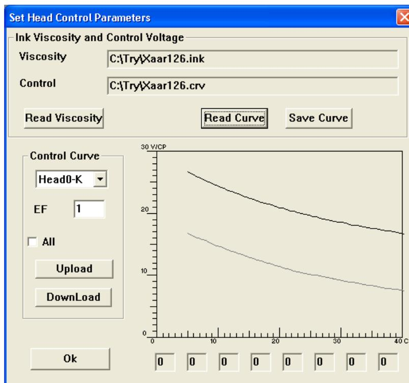
1) **Viscosity file:** Open viscosity file of ink. This curve shows the relationship between viscosity and temperature.
