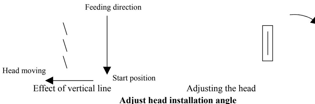
After adjusting the head of color “C”, do the same adjustment to the other heads. During adjustment, do not change “Printer parameter setting”.
