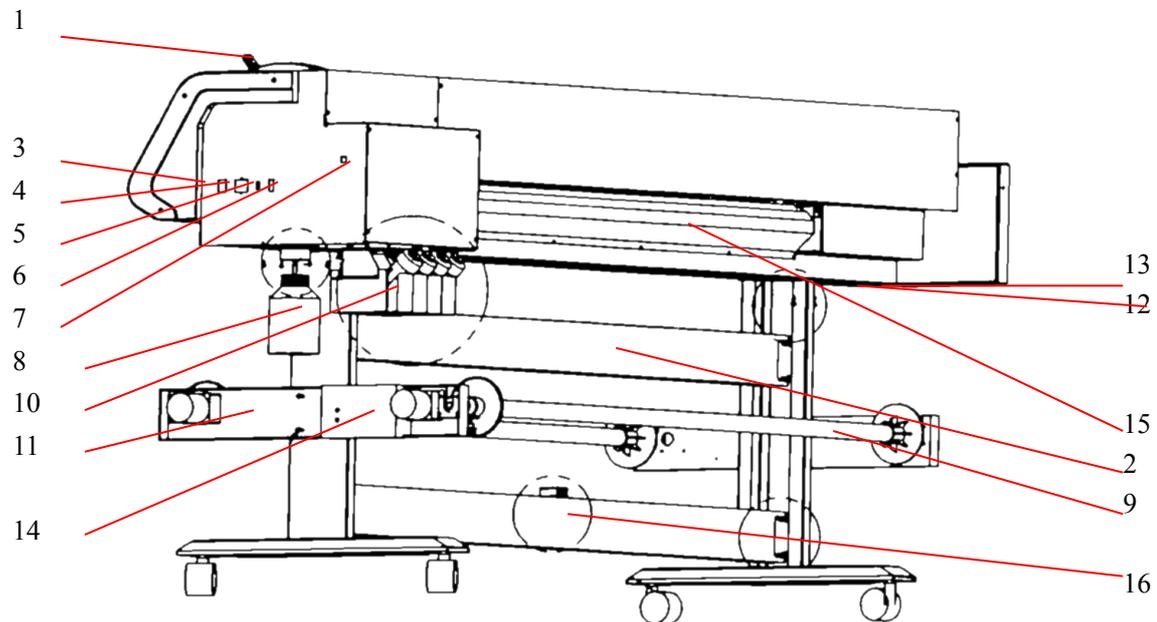
1—wheel controller 2—supporter 3—power switch 4—power port for printing 5—Switch for heating controller 6—leakage protector 7-- port for printing cable 8—waste ink tank 9—media feeding roller 10—ink cartridges 11—media feeding and take-up framework 12—switch for positive pressure clean 13—light switch 14—media feeding control box 15—media 16—media feeding sensor
