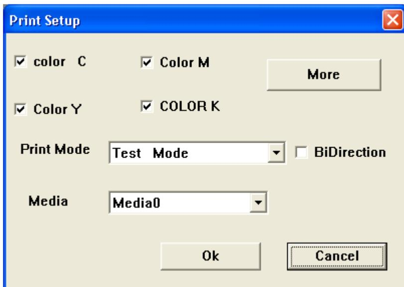
This function is to set the printing parameter, print mode, uni-direction, BID and the color of ink.
