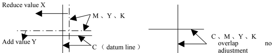
Following above guide to adjust “Head nozzle installation parameter” in “Printer parameter setting”, and input values in the blank behind the distance coefficient. The prior is X, and the latter is Y.
