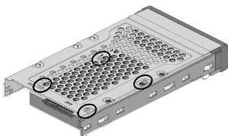
Figure 1-4-1. Installing 2.5-inch SAS/SATA Drive
