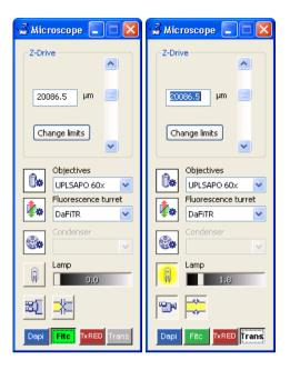
The Microscope dialog window features only those modules that have been configured with the **ObsConfig** software, see Chapter 15.3, Configuring the Microscope. Thus, the contents of the dialog window may differ from setup to setup.
