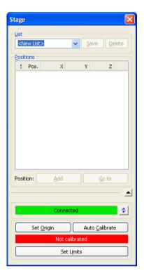
Auto Calibrate. Upon clicking this button the stage will always move to a certain corner position and set this as origin of the coordinate system. The red status box Not calibrated turns green and states Calibrated.
