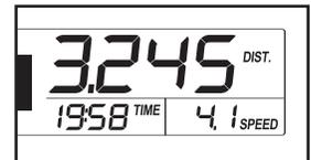
The lower right display can show the speed of the walking belt and the approximate number of calories that you have burned during your workout. This display will also show your heart rate when you use the handgrip pulse sensor.
