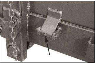
Lubricate Fold Down Side Panel Hinges
