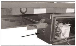
Connect To Battery Charger - Side Mounted Box
