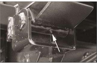
Lubricate Dump Body Pivot Hinges
