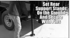
Engage the latch and secure with spring pin. Always secure lock pin prior to operating.
