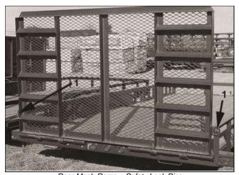
Rear Mesh Ramp – Safety Lock Pins
