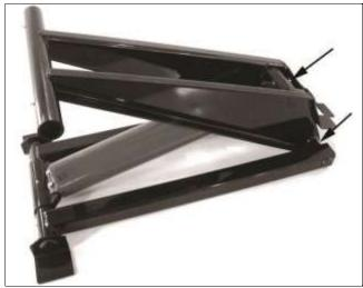
Lubricate Scissor Mechanism
