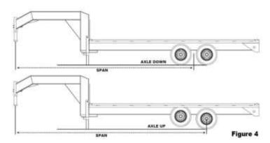
When the front axle is lifted, the rear axle will take on the entire load, which could result in bending or causing other damage.
