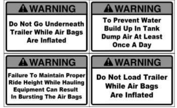
Outside of Toolbox on Trailers Equipped with Air Bags
