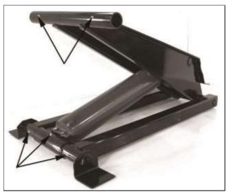
Lubricate Scissor Mechanism
