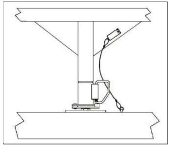
Electric Breakaway Brake Lanyard
