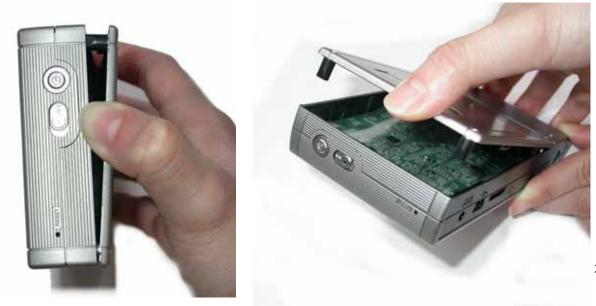
4. To avoid bending the pins, carefully slide the Hard Disk into the chassis.
