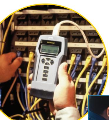
NAVITEK™ is a front-line network navigation tester for anyone who works with both active and passive structured data networks.
