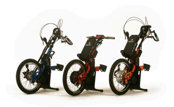
There are three BATEC models: BATEC ELECTRIC, BATEC MANUAL and BATEC HIBRID. All the BATEC models have the same chassis and the same structure, only the transmission system varying in each model:
