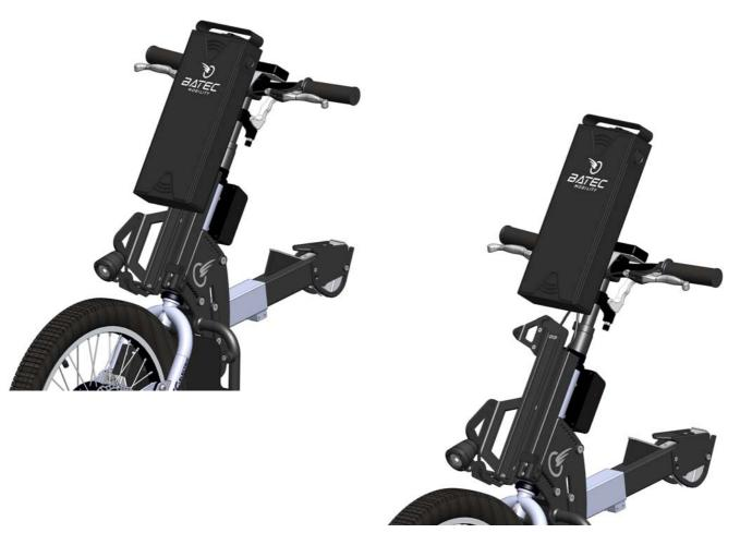
To connect it: Take the battery by the handle. Lean the lower right corner of the battery on the side support tab until it enters the guide. Let the battery slip down slowly along the guide until the lower part is resting fully on the support.
