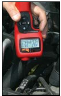
Voltage Display: min / max / average
