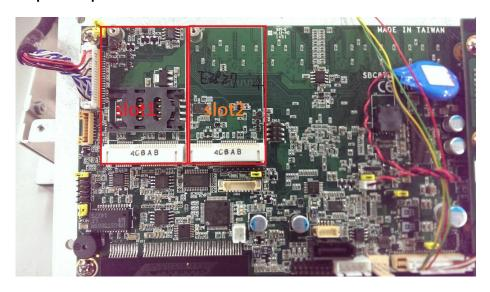
Step 2 Insert the wireless LAN card to the slot. Screw it firmly on the slot.
