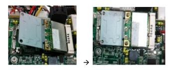
Step 3 There are two connectors on wireless LAN card. One is MAIN, and the other is auxiliary. Connect antenna cable to MAIN connector on wireless LAN card.
