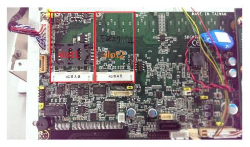
Step 2 Insert the mSATA card to the slot 2. Screw it firmly on the slot.
