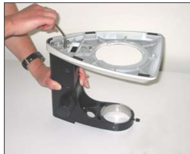
Insert 3 screws from the bottom of the base and screw them tightly
