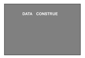
**C.** Make the PTZ controlling device transfer the RS485 data to cctv tester, the hexadecimal signal data will be displayed on the screen as follows, the engineers can analyze whether the data coming from the controlling device is correct or not, or whether it is needed or not by it.
