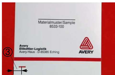
Fig. 2: Punch position = distance of punch center from (inner) edge of material (3).
