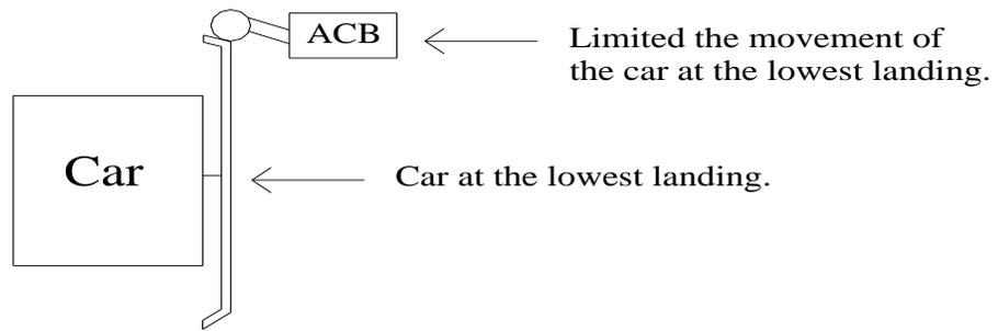
The movement of the car initiated and maintained by the upper access switch. (ACT switch):
