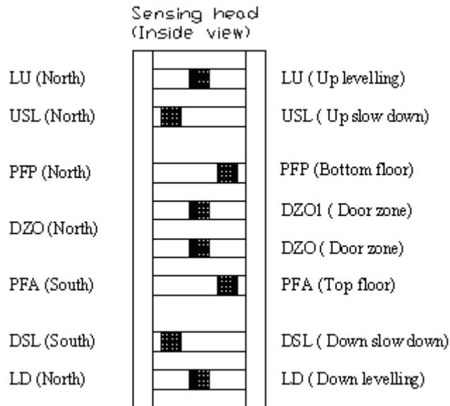
In order to place the magnets in the correct position on the steel tape, it is recommended to bring the car at the exact position where the command has to be energized when choosing an intermediate floor.
