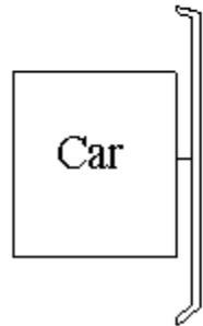
The same corresponding limit switches are found at the bottom floor: LNB, and LEB. The down normal limit switch must be activated as soon as the car goes 1-2 inches lower than the bottom floor.
